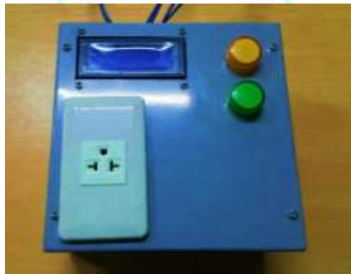
Figure 2: Actual Photo of the Arduino-Based Load Current Display and Time-Delay Protective Device for ACUs
