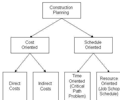
Figure 7: Alternative Emphases in Construction Planning
