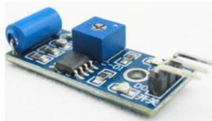
Figure 1: Vibration tilt switch
