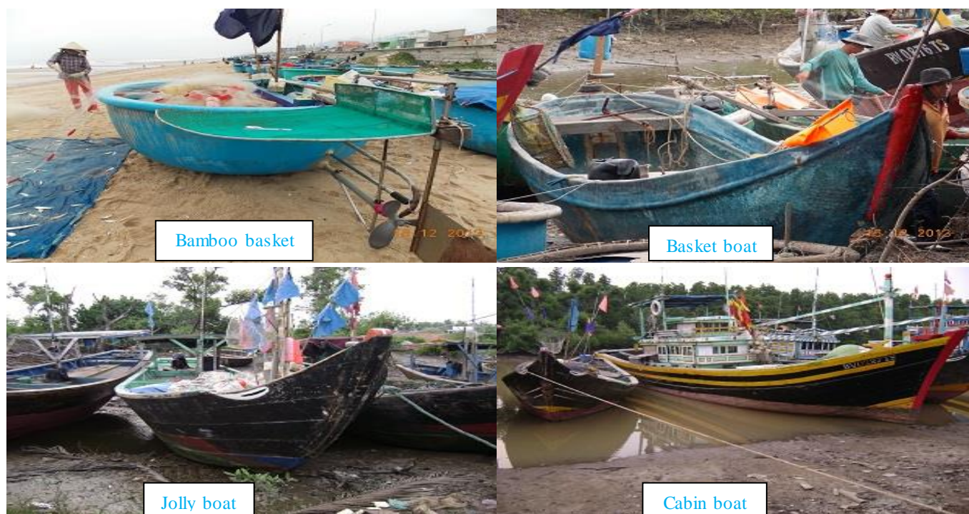
Figure 2: Cabin boat, jolly boat, basket boat, and bamboo basket (Photos: Nguyen Bach Dang, 2013)
