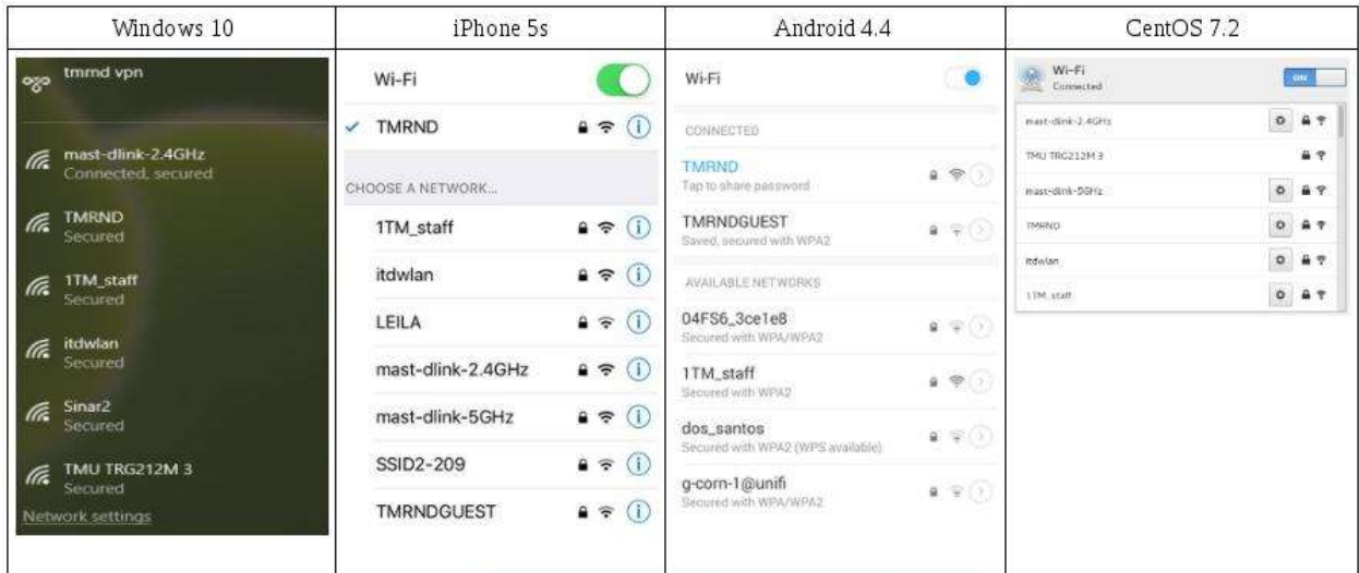
Figure 2: Wi-Fi signal quality indicator on several platforms
