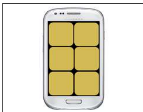
Figure 4: Braille keypad with six buttons
